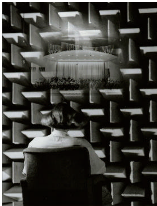
Figure 4.52. A listener in an anechoic chamber experiencing a virtual concert hall. “Auralization is the process of rendering audible, by physical or mathematical modeling, the sound field of a source in a space, in such a way as to simulate the binaural listening experience at a given position in a
