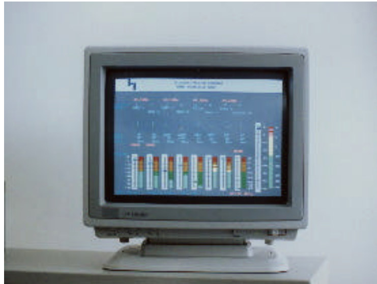
Figure 5.15. The interface for the BMC binaural mixing console manufactured by HEAD acoustics. Courtesy of Sonic Perceptions–HEAD acoustics.
