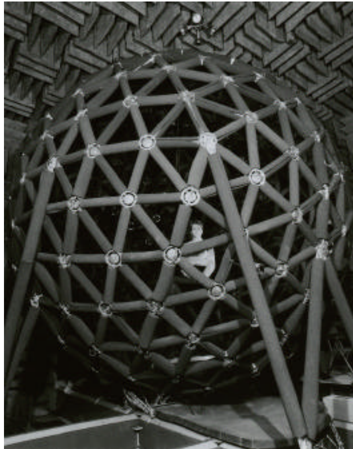
Figure 4.23. The “speaker cage” developed at Armstrong Laboratory, Wright-Patterson Air Force Base for HRTF measurements. Note the sound absorbing foam around the struts. Courtesy of Richard McKinley, Armstrong Laboratory, Wright-Patterson Air Force Base.
