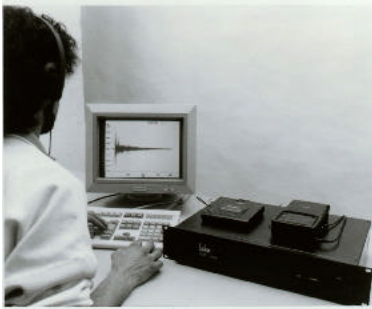
Figure 4.46. Specialized hardware for convolution with long FIR sequences include the Lake FDP1+. The user is playing a reflection-free recording through the signal processor and then digitally recording the output while monitoring the result over headphones. The impulse response of the virtual room is seen on the computer screen; this information can originate from either actual room measurements or room modeling programs.
