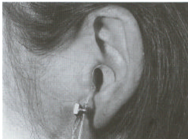
Figure 4.21. Placement of probe microphone in the ear. Courtesy of Fred Wightman and Doris Kistler, University of Wisconsin, Madison; used by permission of the American Institute of Physics.
