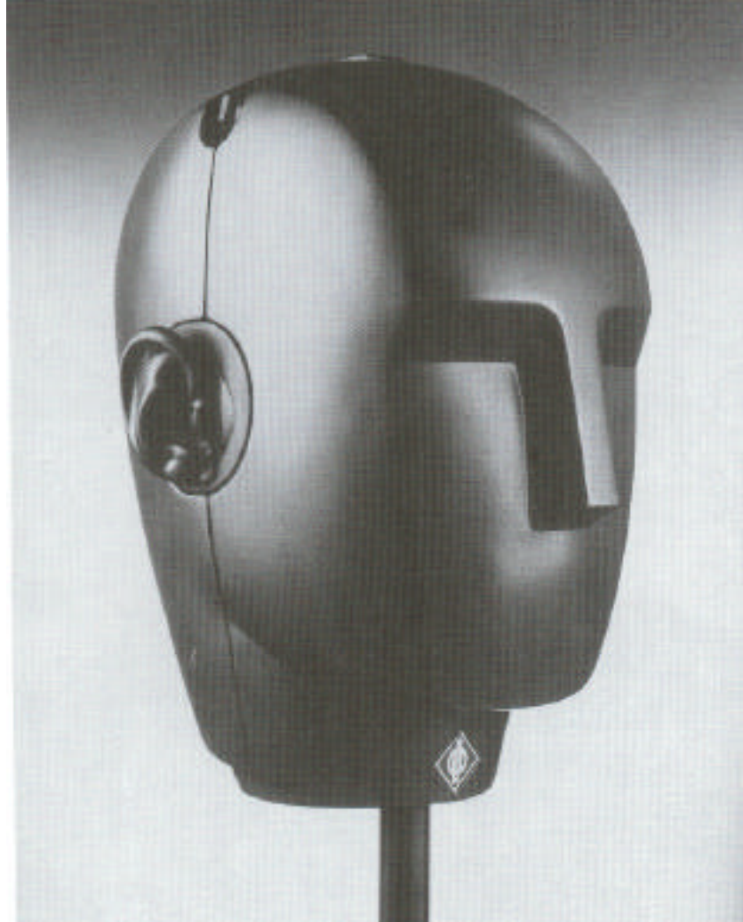
Figure 4.28. The Neumann KU-100 dummy head. This is the third generation of Neumann binaural recording devices (following the KU-80 and KU-81). Photograph courtesy of Juergen Wahl, Neumann USA.
